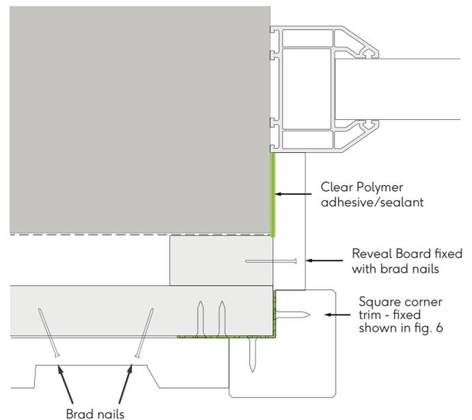
Fig. 15 - Window/door jamb detail - brad nails
