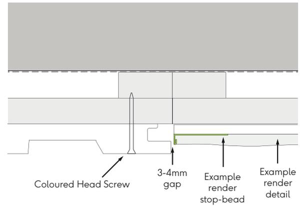
Fig. 19 - Corner profile butting up to render
