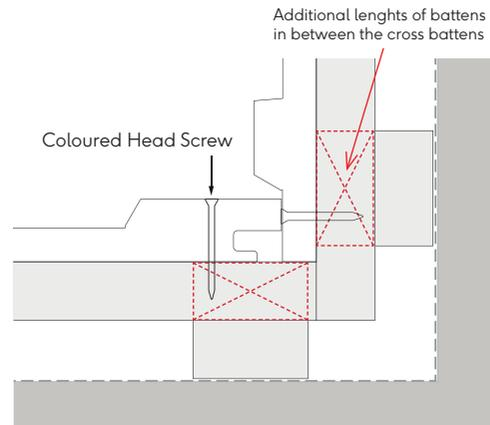
Fig. 9 - Internal butt joint detail
