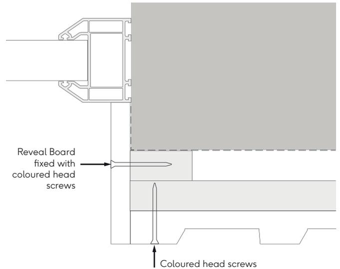
Fig. 13 - Window/door jamb with reveal boards
