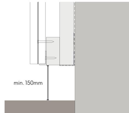
Fig. 4 - Install detail above ground level
