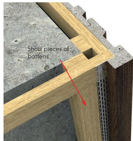
This is to provide fire compartmentation to achieve a Euroclass D and can also be used to offer more support for the corner profile.
