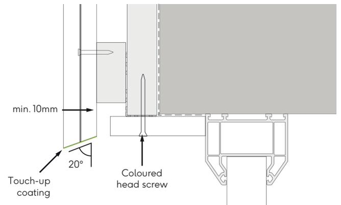
Fig. 14 - Window/door head with angled cut
