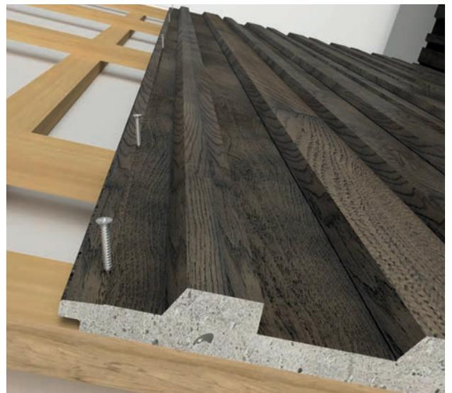
Once the first board has been installed, the second board can be installed beside it, with the groove covering the tongue of the previous board. Check the boards against a level every 4/5th board to ensure that the boards are keeping upright, adjust the spacing between the following boards accordingly if needed.
