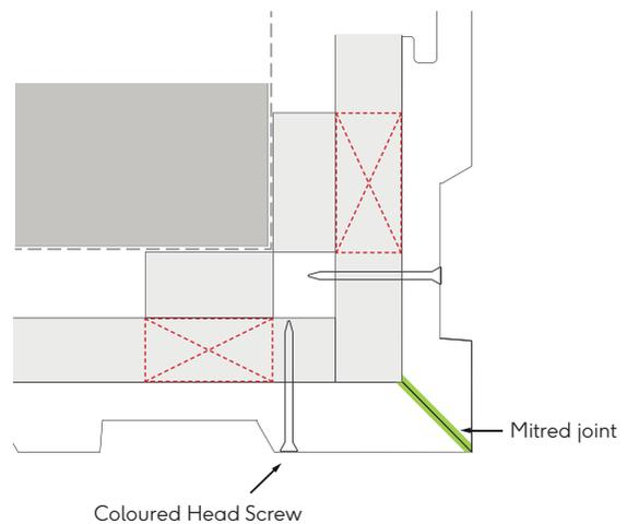
Fig. 10 - External mitred corner detail
