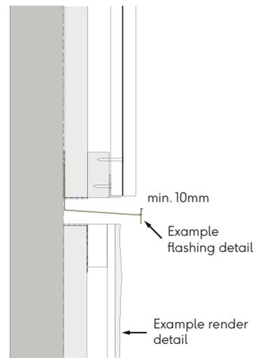
Fig. 21 - Installing cladding above render
