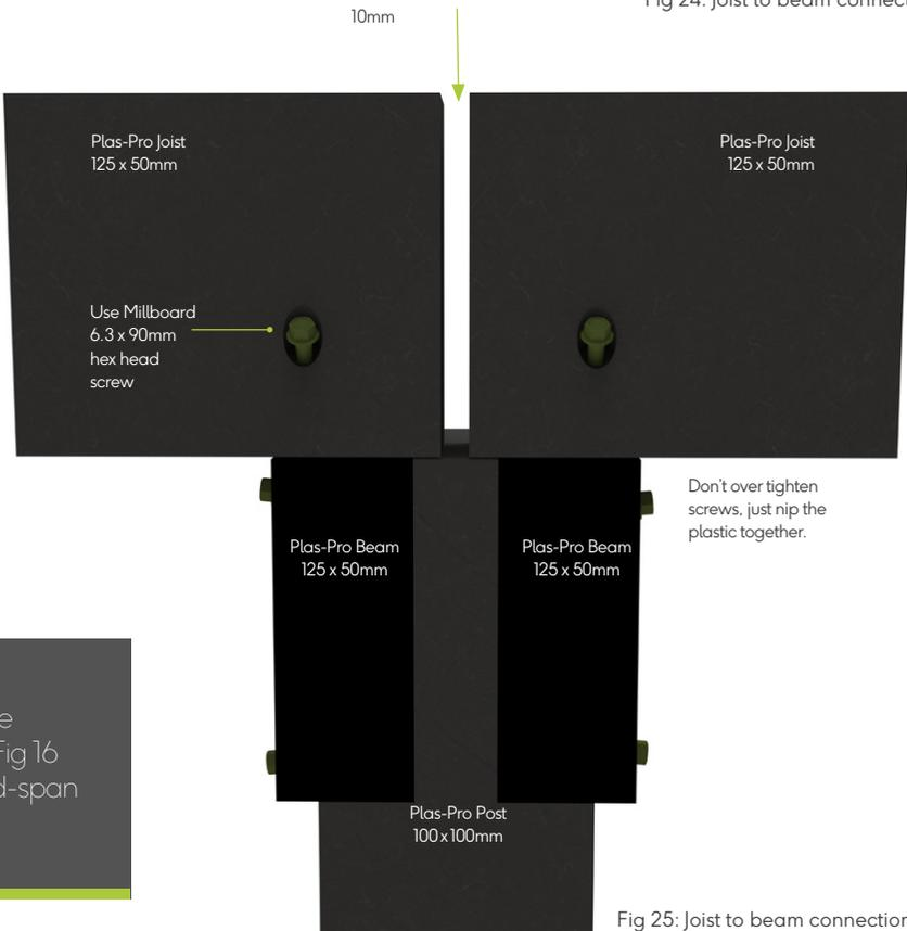
Fig 25: Joist to beam connection
