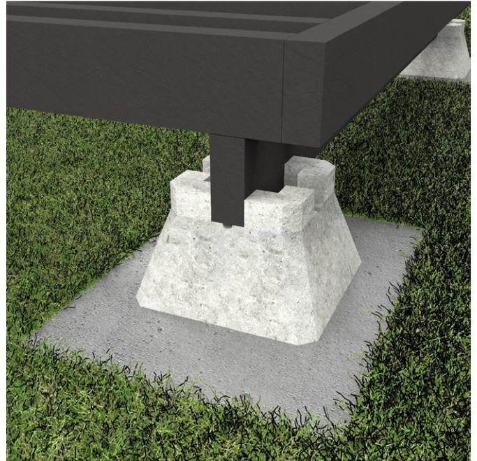
Fig. 15a - Pre-cast concrete pier
