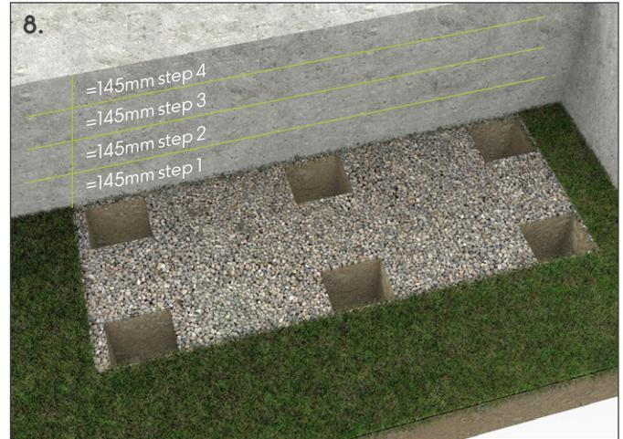
f. 100 x 100mm Posts can be cut to length and fixed in position on the base frame. The 1st row of posts **1** will sit flush with the top of the base frame, the second **2** will sit flush with the top of the 2nd step (in this case 145mm higher), the third **3** will sit flush with the top of the 3rd step (in this case 290mm higher) The front and back rows of posts will protrude 400mm down into pre-prepared post hole positions.
