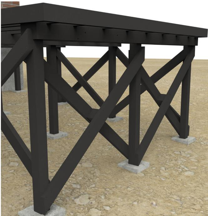
Fig. 10 - Sway/Diagonal bracing
