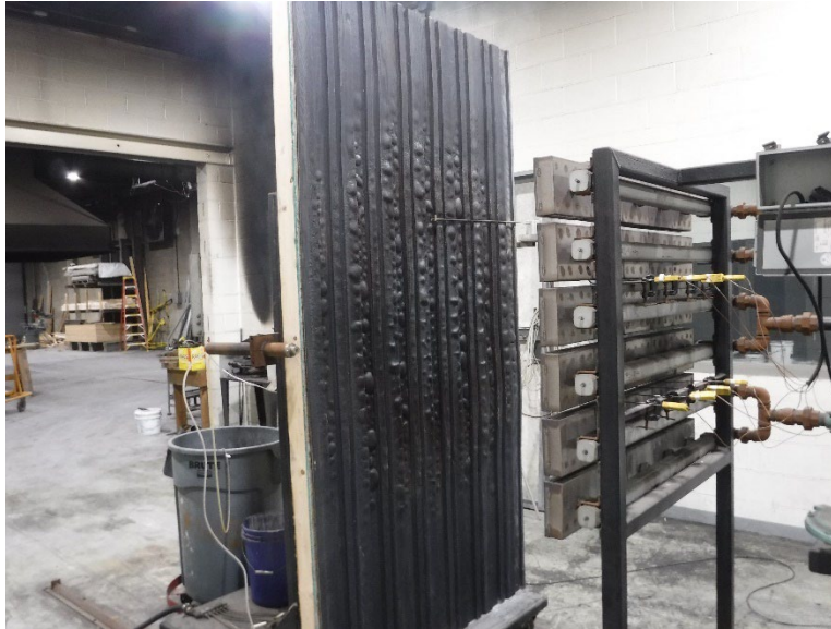
Photo No. 7 Post-test Exterior
