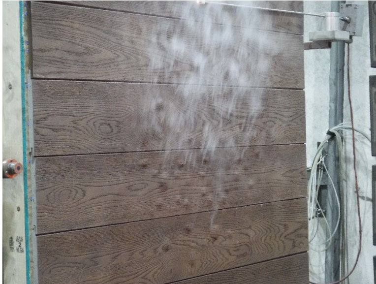
Photo No. 9 Bubbling of Exposed Surface
