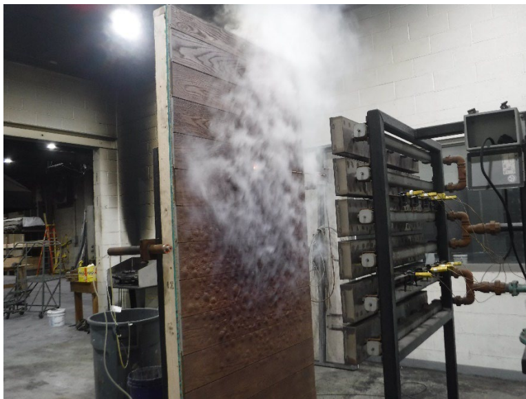
Photo No. 10 Charring of Exposed Surface
