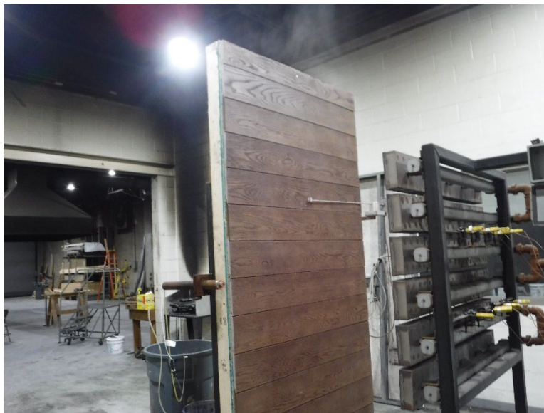
Photo No. 8 Smoke Emitting from Test Assembly
